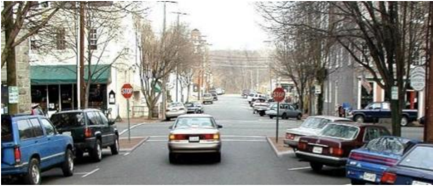
Example of curb extensions. (Credit: Marvel Schmaedick)
